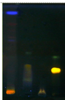
Fig. 3. Chromatogram obtained before revelation (mobile phase B) 1.DPH 2.quercetol, kaempferol (bottom-up); 3.myricetin; 4.luteol
